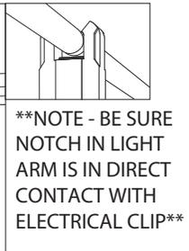
**\*\*NOTE - BE SURE NOTCH IN LIGHT ARM IS IN DIRECT CONTACT WITH ELECTRICAL CLIP\*\***
